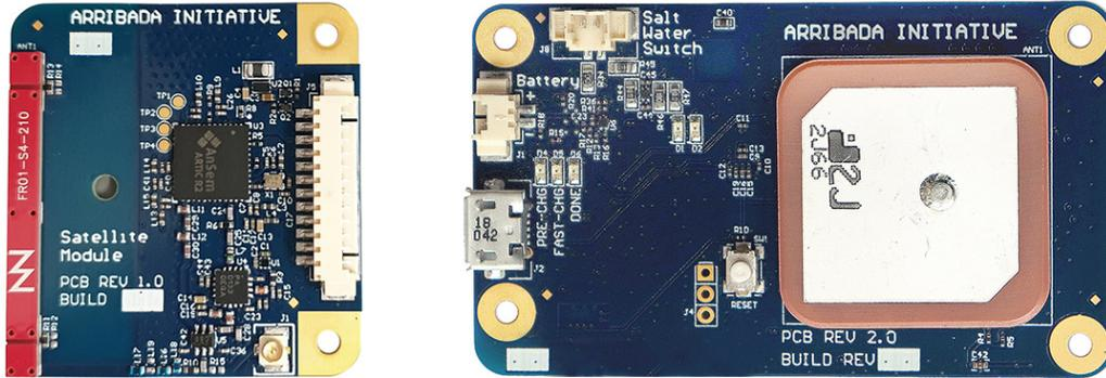
The main Horizon board accepts either an ARTIC R2 module, or a Cellular SARA-U270 module.
