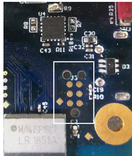
To program the board, once the J-Link debug probe has been connected to the target board as show above, then run the following commands from the arribada\_nrf52840\_tracker root directory:
